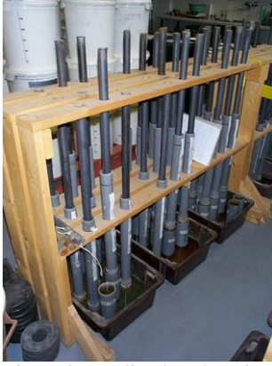
Figure 3. Loading bench and peat specimen samples.
