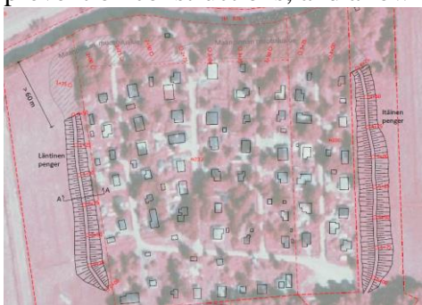
Figure 7. Pirttiranta – the location of the flood dikes (Vantaa).
