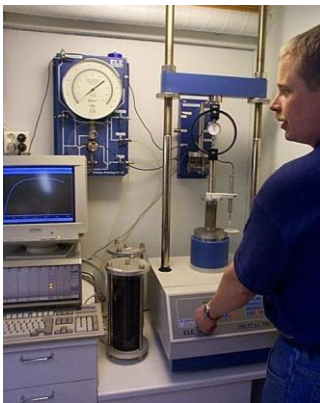
Figure 4. Unconfined compressive test in progress. Ramboll Finland Oy.
