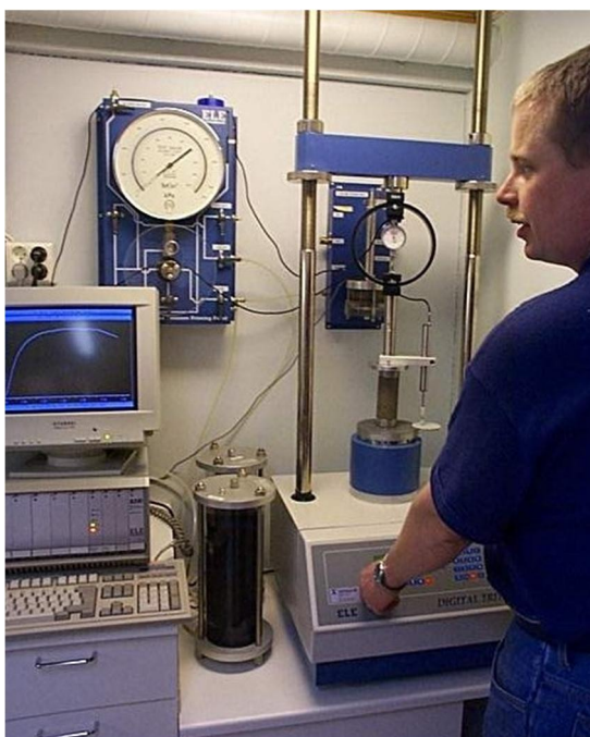
Figure 2. Unconfined compressive test in progress. Ramboll Finland Oy.
