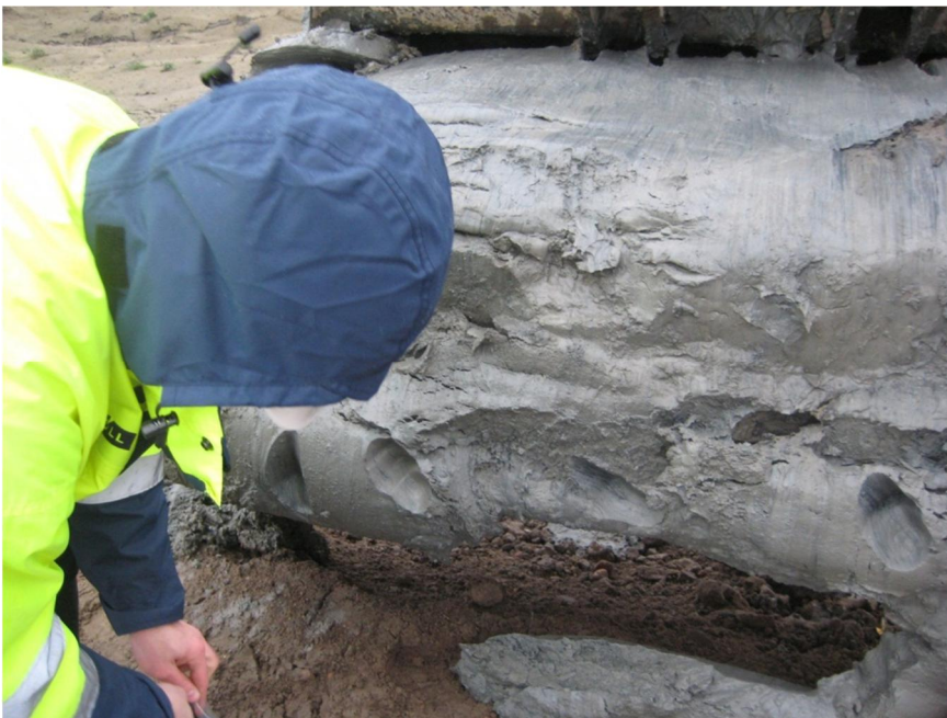
Picture 12.12 Dredged sediments before stabilisation.
