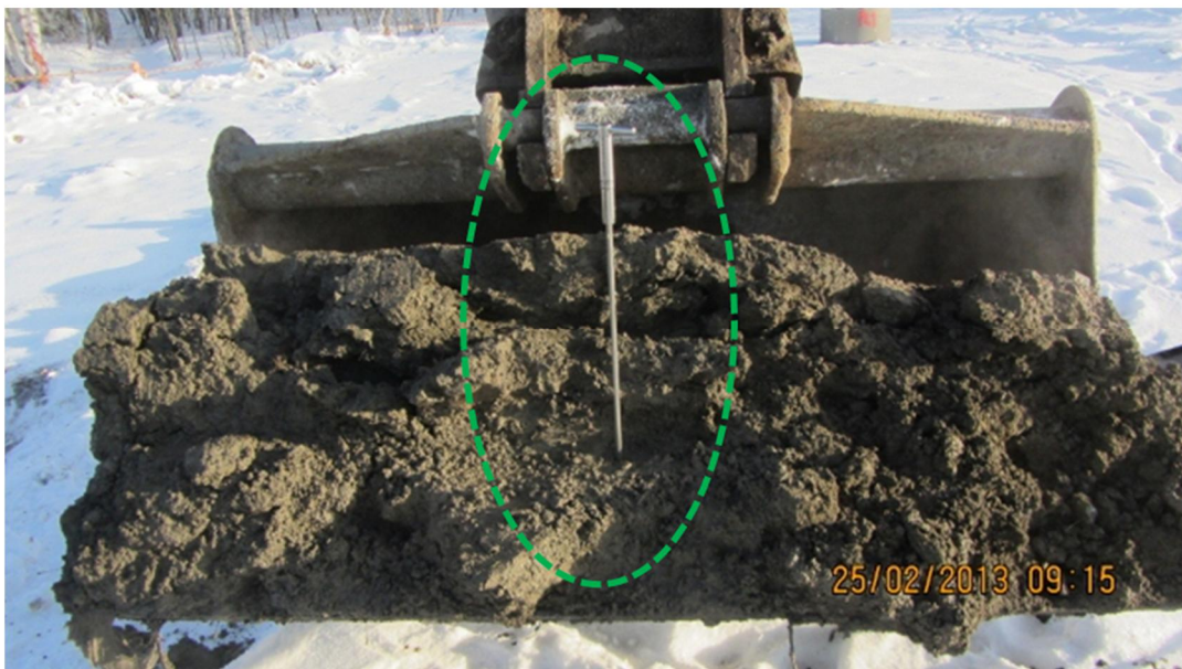
Figure 7.8 Hand held vane shear test apparatus a) source: ( www.esands.com ) b) testing in the field
