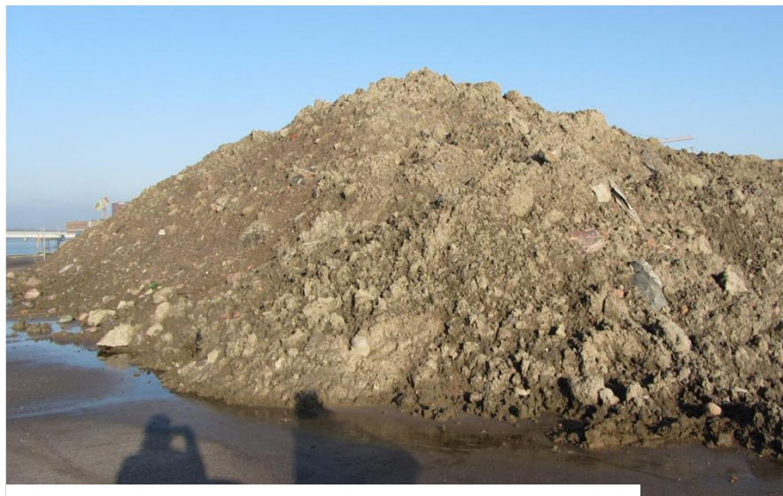
Stabilized material on stockpile
