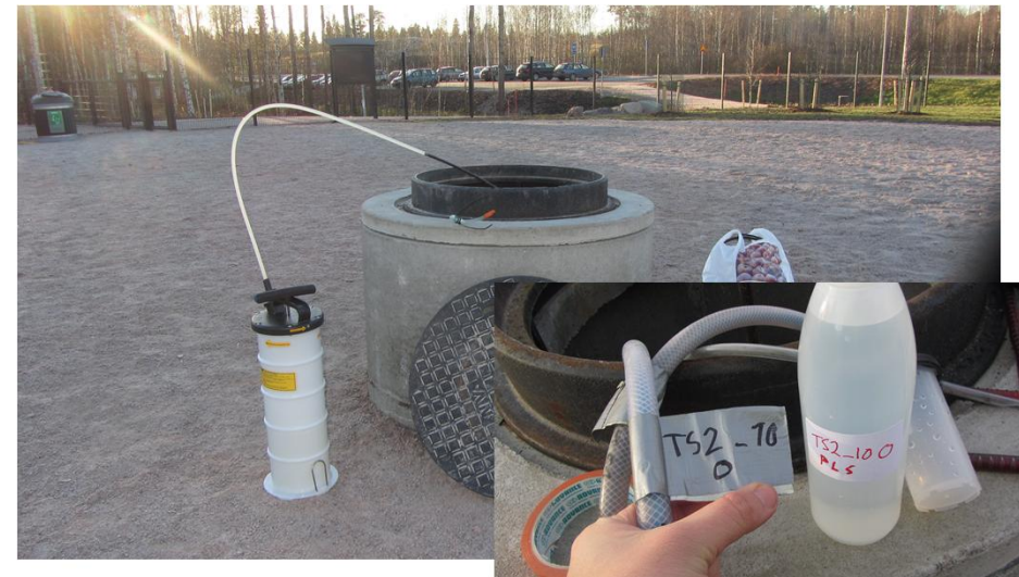
Measuring lysimeter in ready Dog Park 12.2.2012
