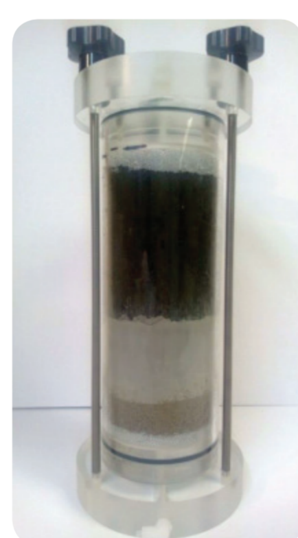
Figure 1. The sample packed in the column before starting the test. The materials starting from the below are moraine, gold enrichment sand and nickel enrichment sand. In both ends of the column is placed 1 cm layer of inert glass pearls.
