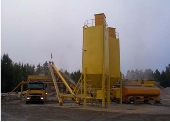
Production of the fly-ash binder admixtures. A new type of mixing station
