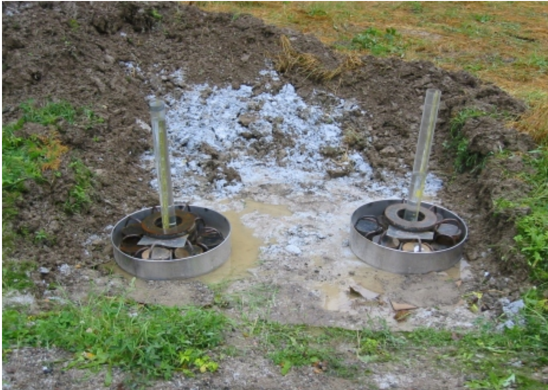
Figure 12. Pilot 2003. Infiltrimeter measurement done in the fibre clay groundwater structure.
