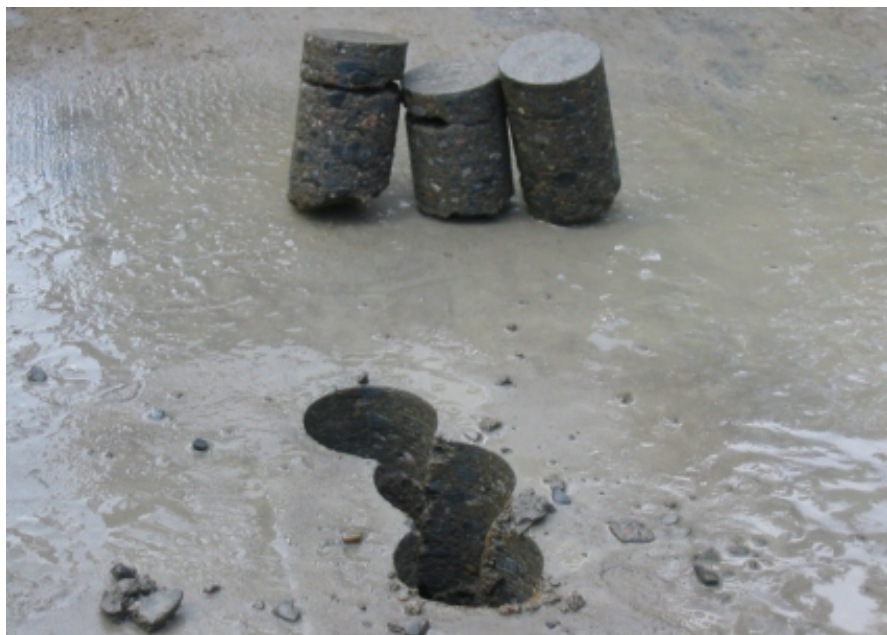
Figure 5. Pilot 2002. Drilled samples from a stabilised section.
