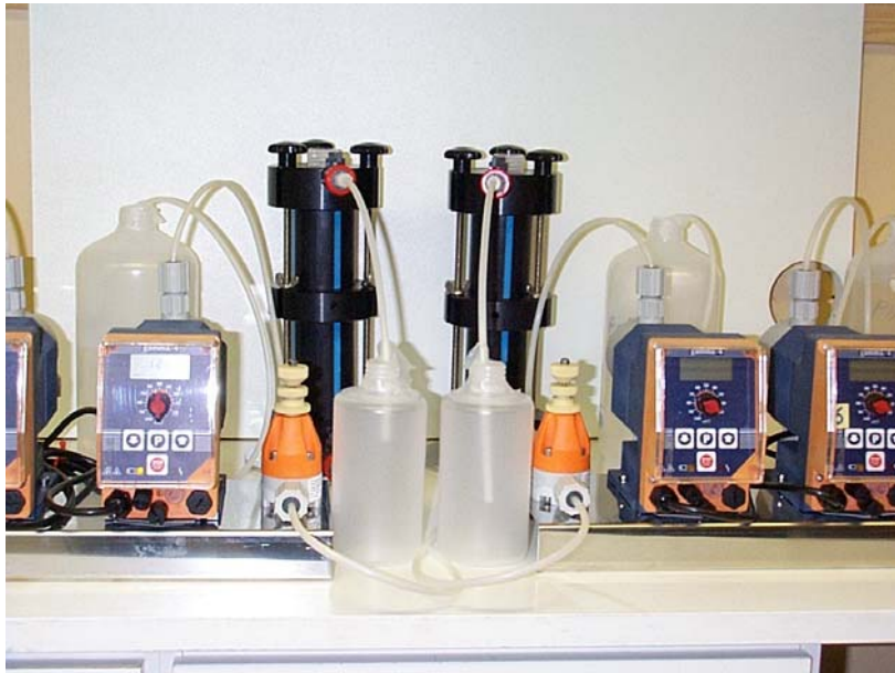
Figure 4: Column test. Leaching test according to NEN7343. SCC Viatek Ltd, SGT.
