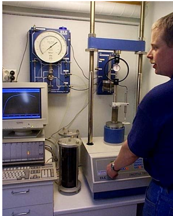
Figure 1: Unconfined compression test in progress. SCC Viatek Ltd, SGT.
