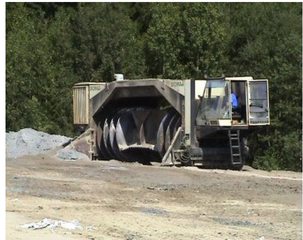
Figure 5: Stack mixer used for the mixing of fibre-ash in 2003.
