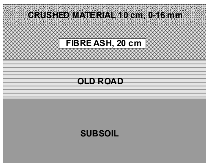
Figure 14. Cross section of the fibre-ash structure for Pilot 2003
