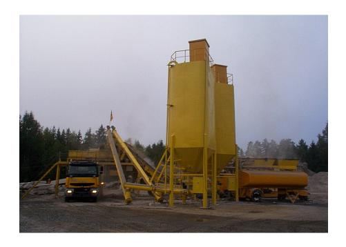
Figure 2: Mixing station for binder admixtures
