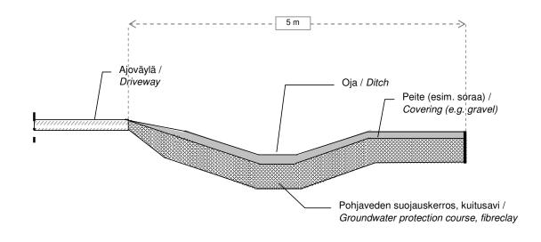
Figure 12: Principle of the gw-protection
