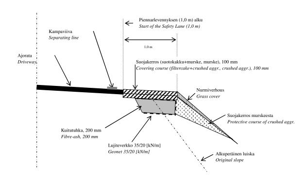
Figure 19: Principle of the safety lane structure
