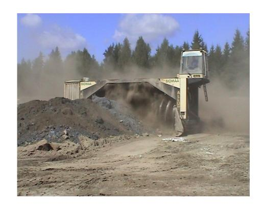
Figure 8: Stack mixing of the fibre-ashes
