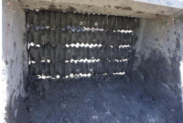
"Process stabilisation" - screener crusher (ex-situ)
