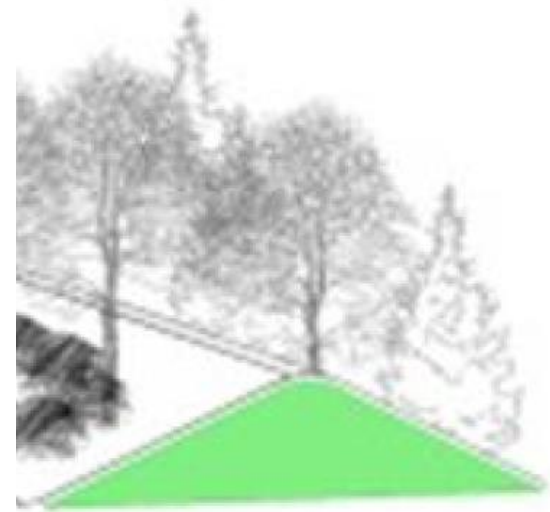
Solidification of contaminated sediment or soil masses in harbour or in noise barriers (etc.)
