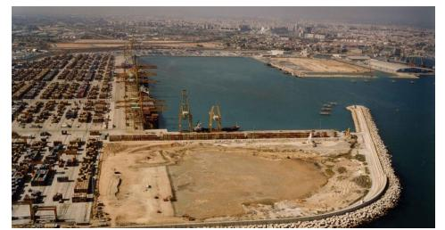
Mass stabilization area on the left and dredged sediments before stabilization on the right.
