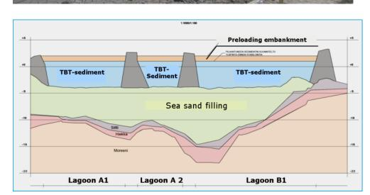
The principle of utilizing sediments in Vuosaari.
