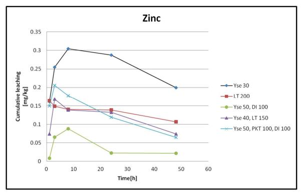
There are differences between binders during the first 10 hours of the test, but after that the differences start to reduce and the leaching of zinc continues to decrease (total content of the zinc in the sediment sample is 560 mg/kg)
