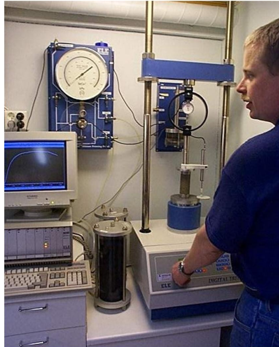
Figure 1 Unconfined compressive test in progress. Ramboll Finland Oy.
