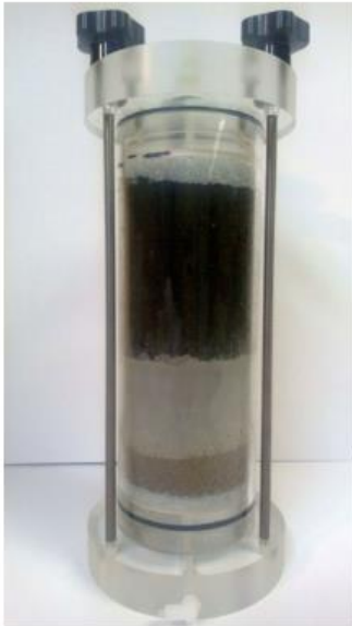
Figure 1. The sample packed in the column before starting the test. The materials starting from the below are moraine, gold enrichment sand and nickel enrichment sand. In both ends of the column is placed 1 cm layer of inert glass pearls.
