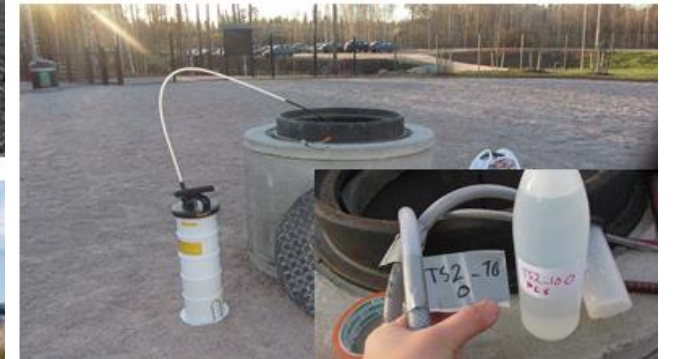
Measuring lysimeter in ready Dog Park 12.2.2012
