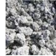
Fibre clay (deinking sludge)
