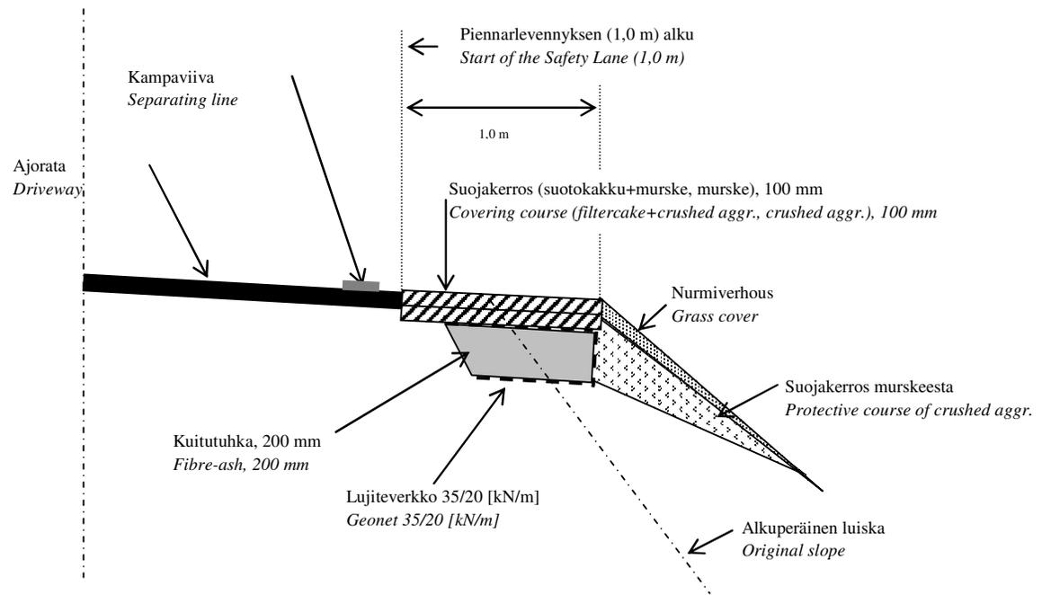
Figure 19: Principle of the safety lane structure
