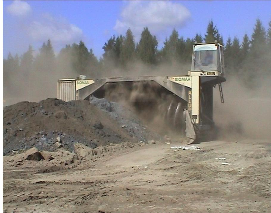
Figure 8: Stack mixing of the fibre-ashes
