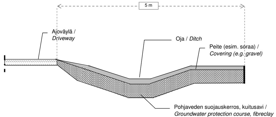
Figure 12: Principle of the gw-protection
